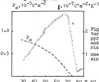
Fig. 1. The temperature dependence of pyrocoefficient  $\gamma$  (T) and spontaneous polarization  $P_s(T)$  for 1 one of chiral synthesized polymers.
